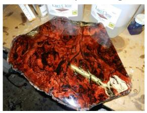
Burl with many open cracks filled with LuciClear before machining into a bowl.
